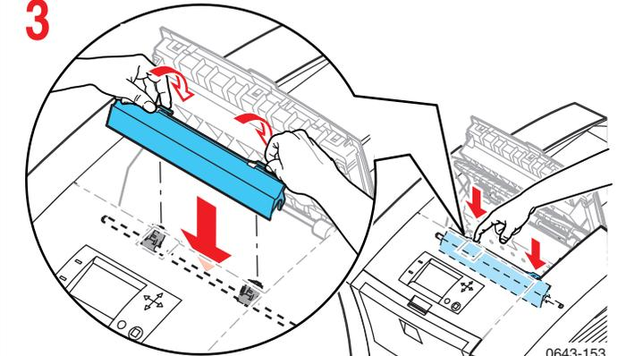
◆ Open the exit cover to access the rapid-release guide.
